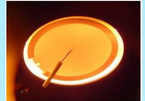
2 inch diameter Inconel disc at 975°C with TC for calibration.
